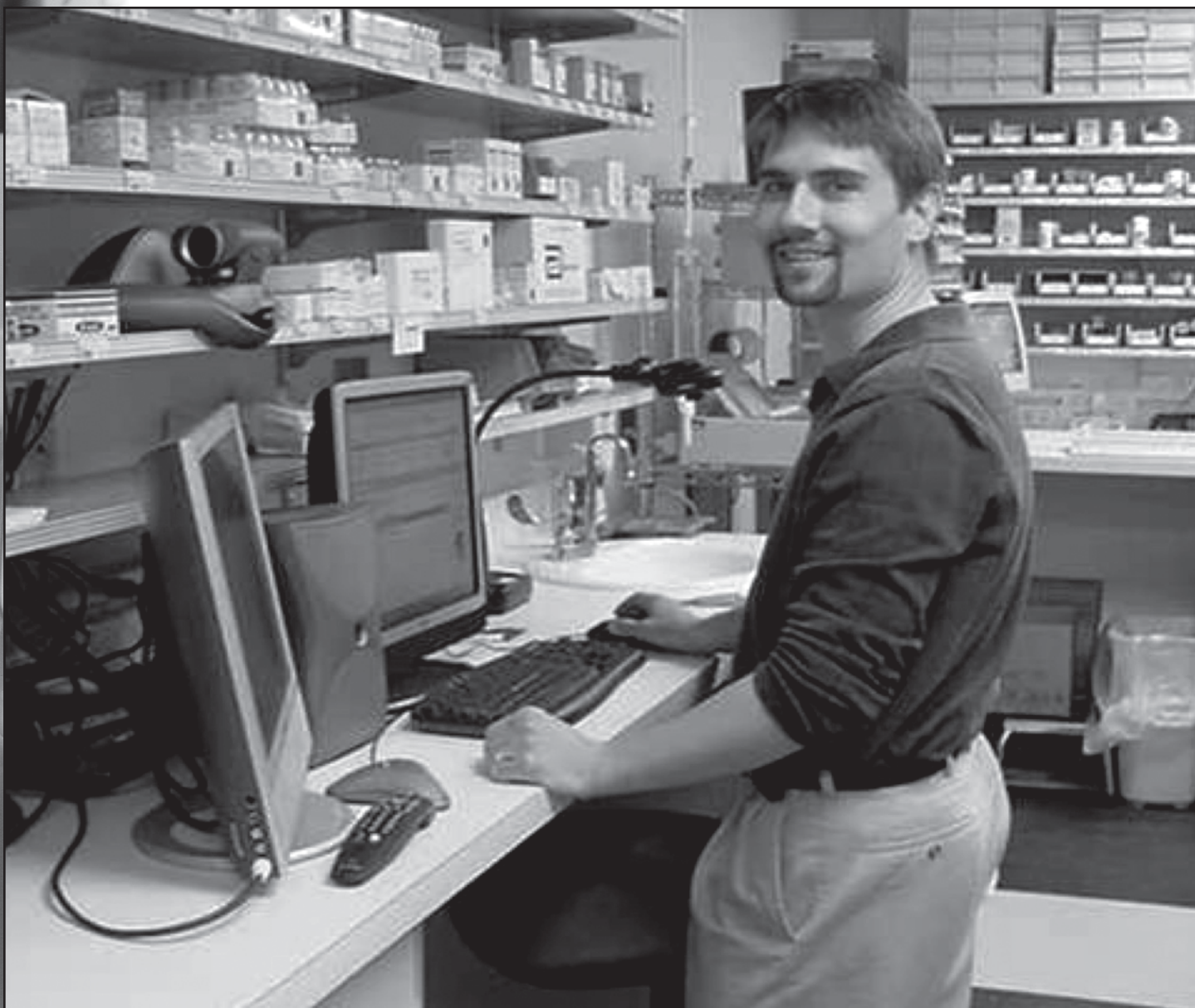
A typical hospital telepharmacy equipment set-up includes audio and video computer links and document cameras to allow a pharmacist at a central pharmacy site to visibly and verbally supervise a pharmacy technician at a remote rural hospital site to process medication orders.
